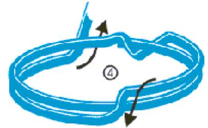
**5. - When you get back to the node, loop the wire through the center again.** It is not necessary to use glue at each revolution, but it is generally a good idea to glue the first wrap in place, that way the circle will stay the same size as you wind the coil. Otherwise, it will try to unravel itself.
