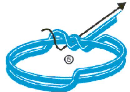
**6. - Continue winding the coil, repeating steps 1 through 5, as shown.** When you run out of cable, use a little glue to hold the end of the cable in place.
