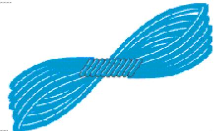
**Just keep wrapping the cable around itself as you go around the circle.** Remember to cross the wire over from the top to the bottom as shown. With a little practice, you will find that the windings form a pattern, and if you make a mistake it will be obvious as it does not fit the pattern. If you are winding this coil around a core, it is even simpler, because all you have to do is keep feeding the end of the wire between the coil and core, once for each revolution.
