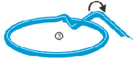
**4. - Opposite the node, cross the wire over from the top to the bottom as shown.**
