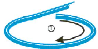
**2. - When you complete the first wrap, feed the wire through the center of the circle** so it wraps around itself as shown. Use a little glue (hot melt or silicone preferable) to hold the wire in place where it crosses over itself.
